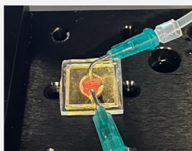
Fig. 2. Microfluidic flow cell attached on top of the nanophotonic SPR sensor chip to deliver sample solution to the chip's sensing area
